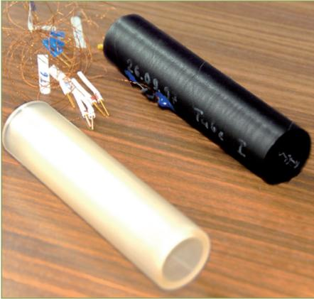
FIG. 16: ZERODUR AND CARBON-FIBER REINFORCED PLASTIC TUBES.
