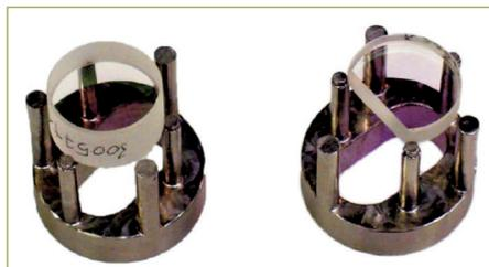
FIG. 6: MEASUREMENT MIRROR (LEFT) AND REFERENCE MIRROR (RIGHT) MOUNTED ON THE CLAMPS. THE REFERENCE MIRROR IS CUT IN ORDER TO ALLOW THE MEASUREMENT BEAM TO PASS TO THE MEASUREMENT MIRROR.
