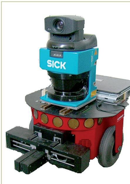
ABB. 3: PIONEER-2 ROBOTER
