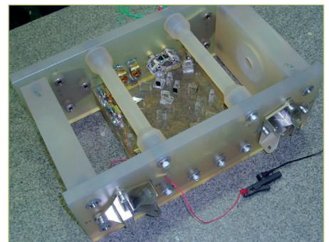
FIG. 1: ENGINEERING MODEL OF THE OPTICAL SETUP FOR LISA PATHFINDER. THE INTERFEROMETER IS REALIZED USING HYDROXIDE-CATALYSIS BONDING TECHNOLOGY.
