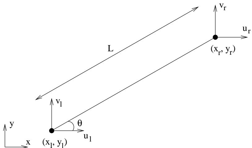
$$\begin{aligned}\cos \theta &= \frac{x_r - x_l}{L} \\ \sin \theta &= \frac{y_r - y_l}{L} \\ L &= \sqrt{(x_r - x_l)^2 + (y_r - y_l)^2}\end{aligned}$$
