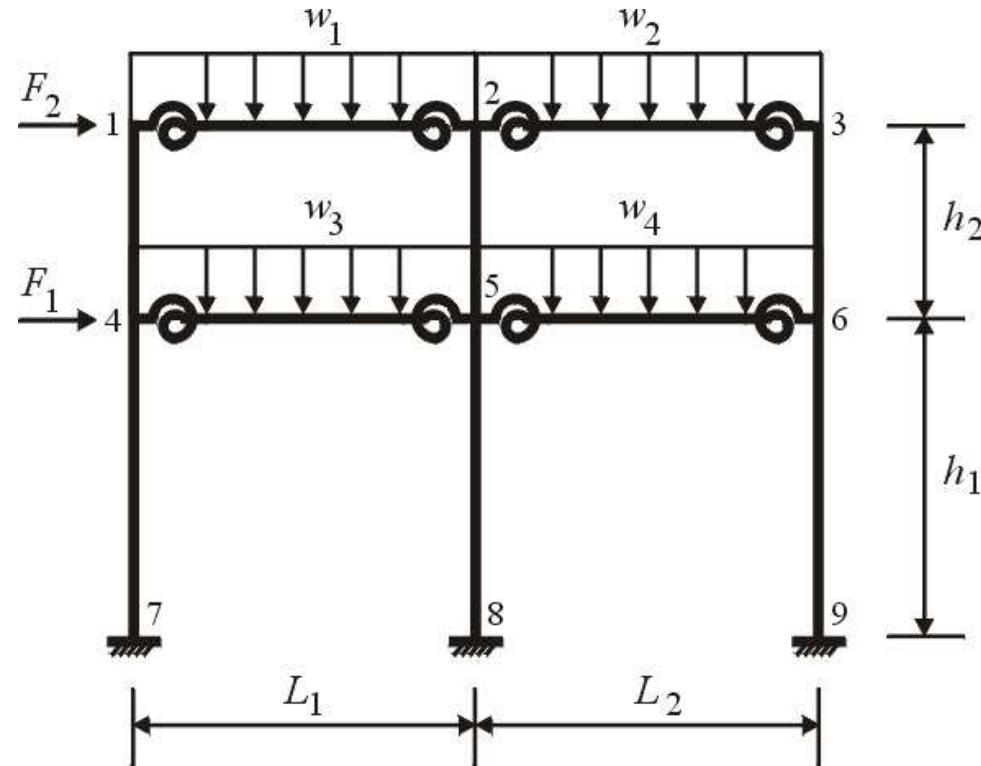
Example: Parametric linear system of order 18 with 13 uncertain parameters
