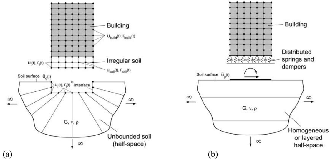
Figure 3. Models for soil-structure interaction; (a) SBFEM model (Radmanovic and Katz 2010); (b) DSD model
