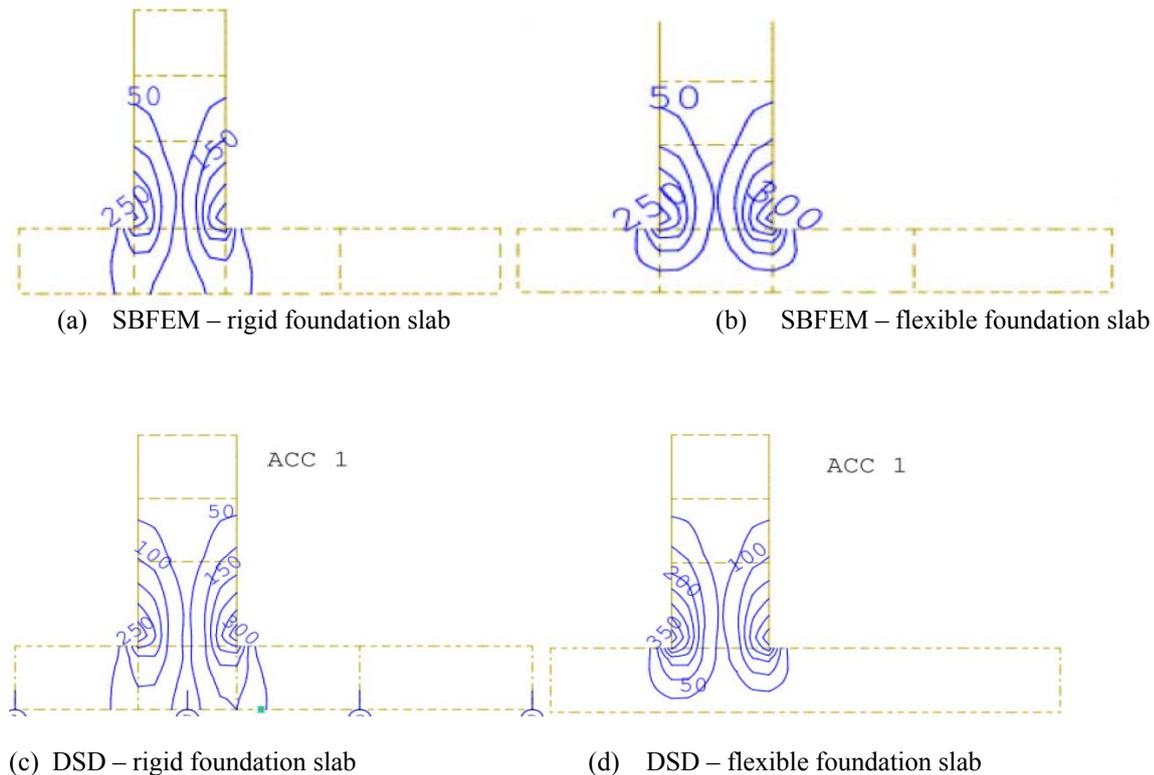
Figure 10. Vertical stress resultants [kN/m] at the bottom of wall W1
