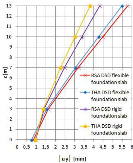
(c) Displacements, model with 5% damping
