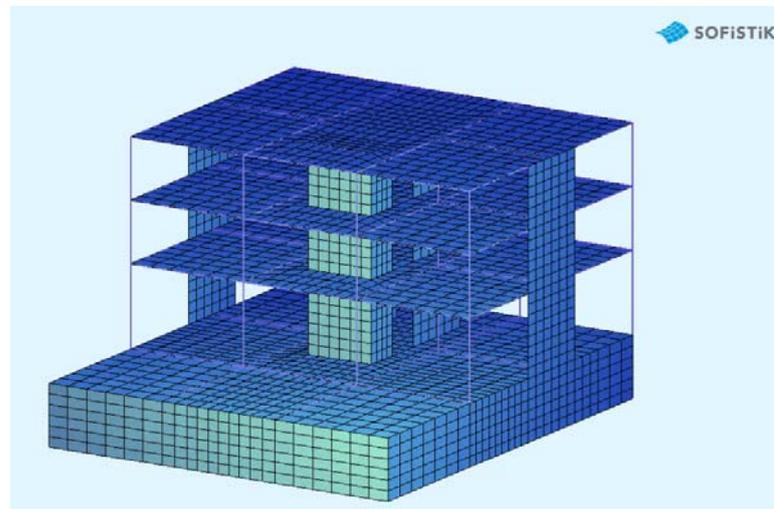
Figure 4. Three-dimensional finite element model of a multi-storey building (Volarevic, 2013)
