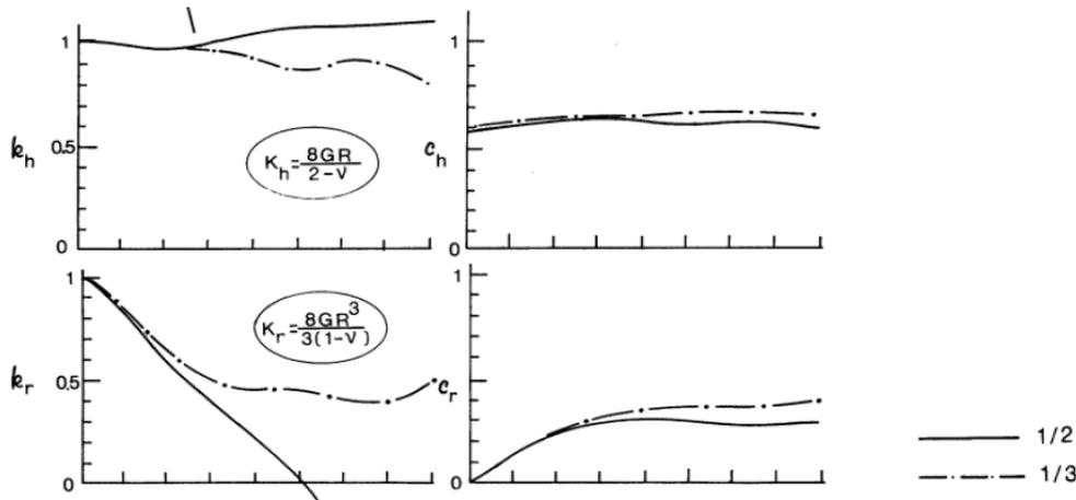
Figure 2. Impedance functions of an elastic half-space for  $\nu = 1/3$  and  $\nu = 1/2$
