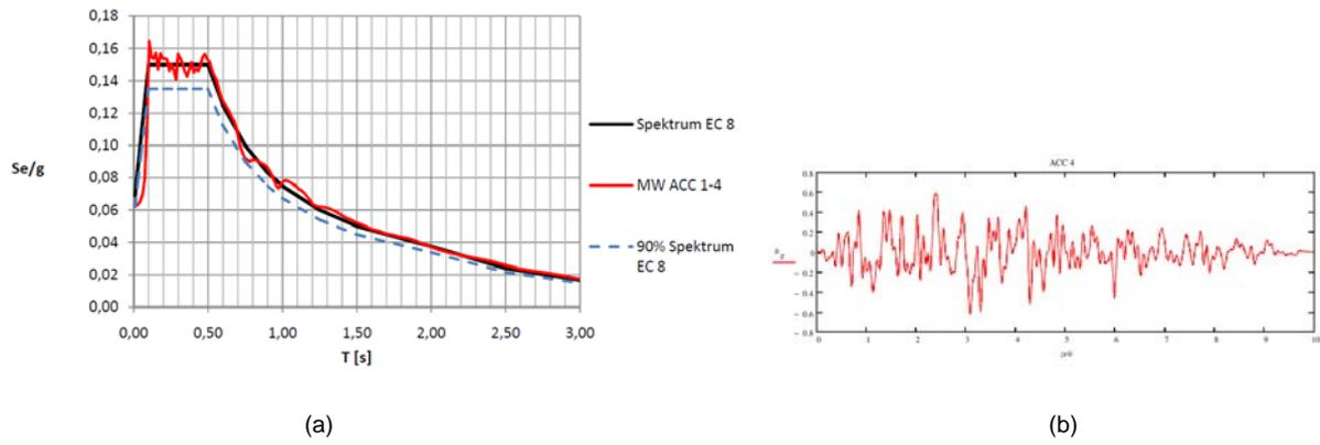
Figure 7. Earthquake action (a) Acceleration response spectrum (b) Time history
