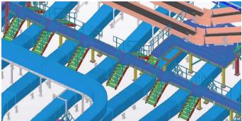
Robert Bird Group utilized BIM and Tekla Structures to model and detail the supporting steel structures for 27 kilometers of baggage handling systems, enabling coordination with other trades and thereby a clash free model.
