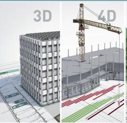
A computer model of a building containing the location-, geometry-, property- and attribute information of its building components (commonly referred to as Building Information Model) A computer model that integrates information of building components with the respective start and finish times of their construction.
